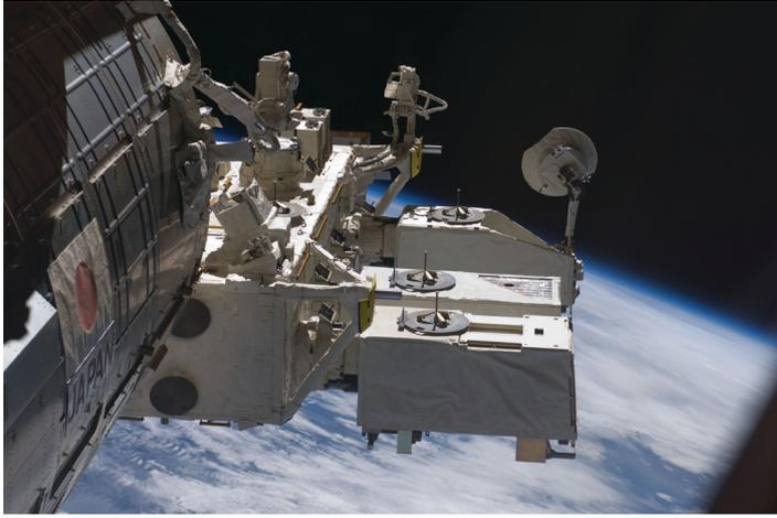
Photo: A picture taken from the Pressurized Module (PM), a part of the Japanese Experiment Module (JEM). SMILES is attached to the Exposed Facility (EF), and sits on the second slot from the front. (Photo courtesy of NASA.)
