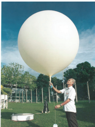
Figure 23: A photograph of the Tai Seng site in Singapore (taken from MSS, 1995). An observer is releasing a weather balloon with attached Vaisala RS80-15N radiosonde (winds from OMEGA global navigation system).
