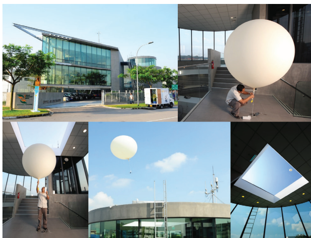
Figure 24: The current Upper Air Station within the 4-story building sharing with the Centre for Climate Research Singapore (CCRS) located at 36 Kim Chuan Road in the central-to-eastern part of Singapore. Top left: The front view of the building; on the top right of this photo, we see the “Launch Platform” where the radiosonde preparation and balloon inflation and launch are conducted. Top right: The inside of the “Launch Platform.” (The radiosonde instrument is prepared at the lower level. See Figure 26.) Bottom left: Just before balloon launch, the ceiling is being opened. Bottom middle and right: Just after a balloon launch.
